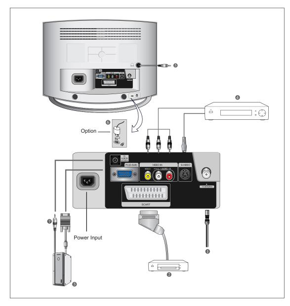
Whenever you connect an audio or video system to your set, ensure that all elements are switched off. Refer to the documentation supplied with your equipment for detailed connection instructions and associated safety precautions.
